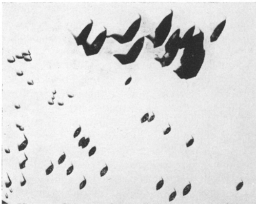
Figure 8 (a) shows pits on \{1100\} plane and (b) shows same area after chemical polishing and re-etching. [0001] direction lies along length of pits from bottom left to top right ( \times 175 ).
